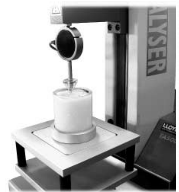
Cone probe shown with TG/BEC back extrusion cell (not included)
